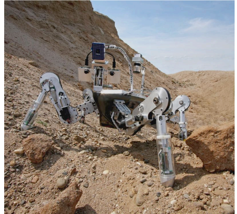
Legged robots Lauron I, II, III, IV (FZI)
